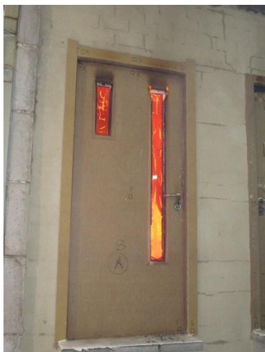
-Time 60 min. Sustained flame doorset B-
