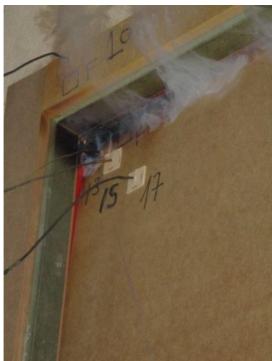
-Time 49 min, Incandescent doorset A-
