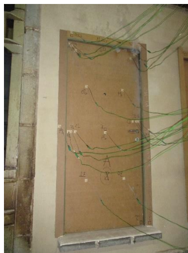
- Time 4 min, smoke output Doorset A-
