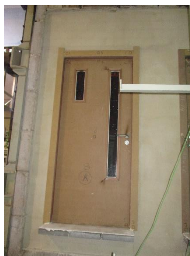
- Time 13 min. Darkening upper zone glasses doorset B -
