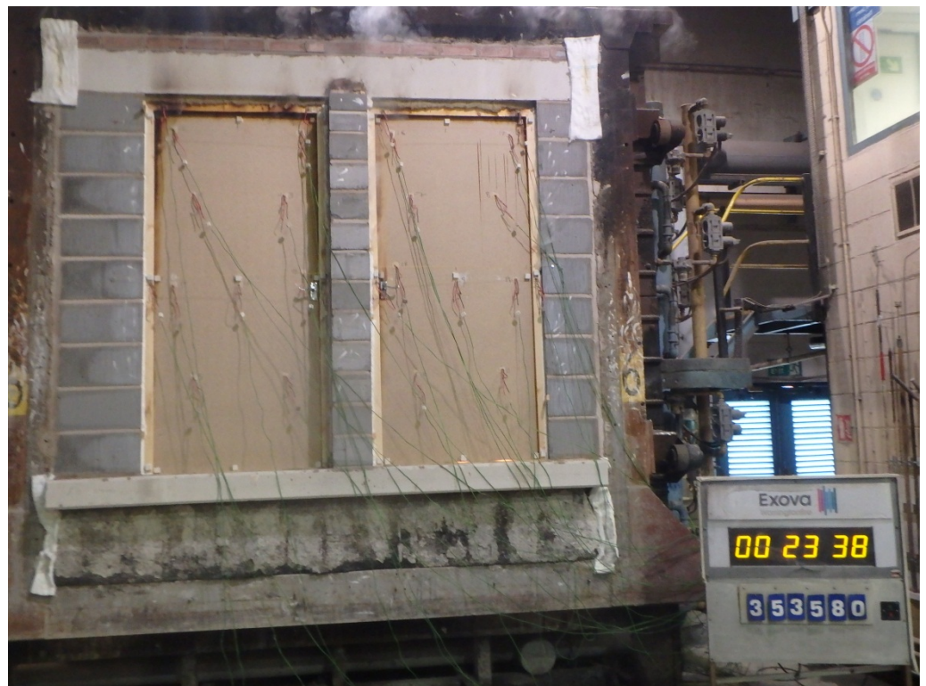
The unexposed face of the Doorsets after 23 minutes of testing
