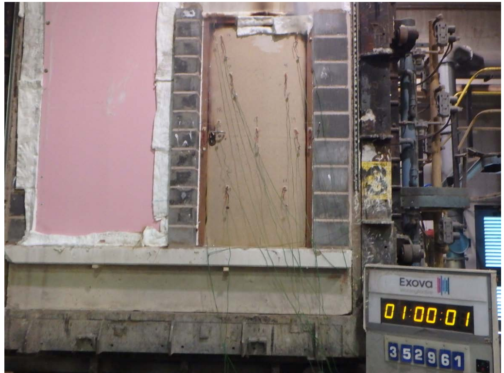
The unexposed face of Doorset B after 60 minutes of testing
