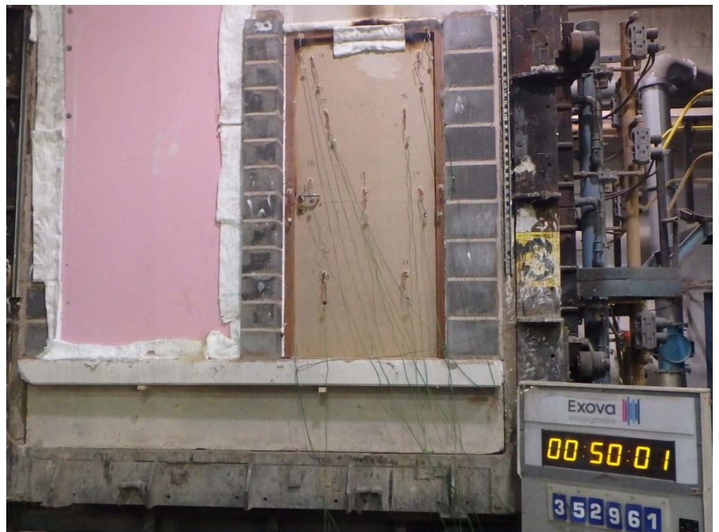
The unexposed face of Doorset B after 50 minutes of testing
