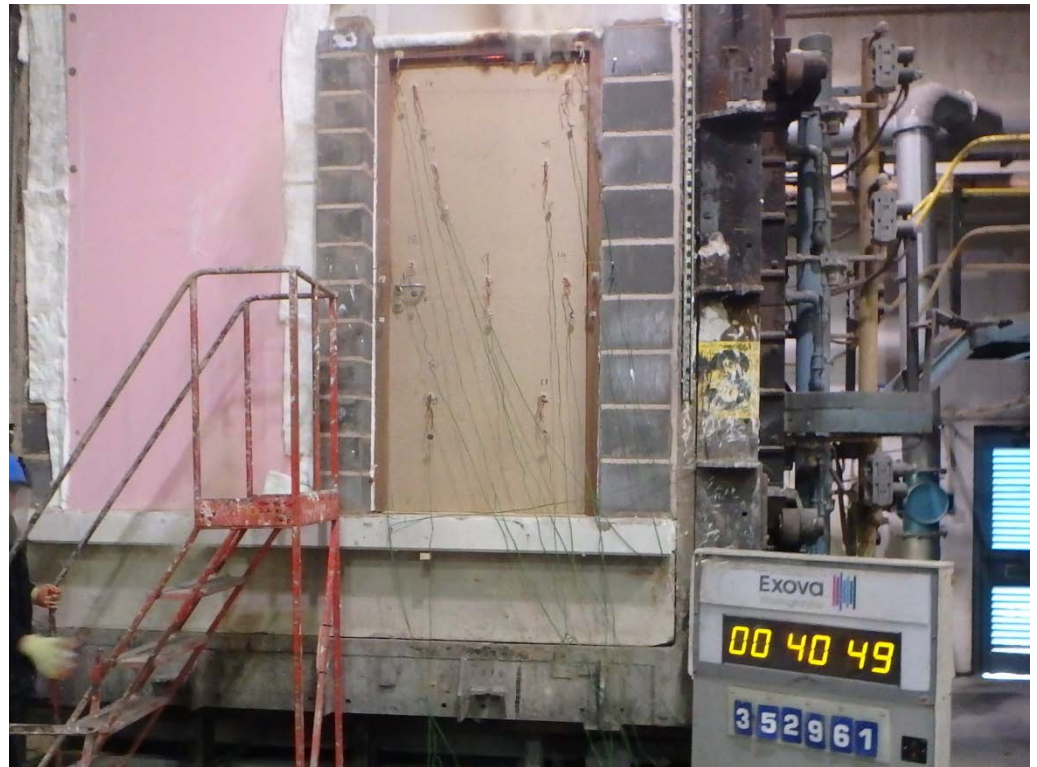
The unexposed face of Doorset B after 40 minutes of testing
