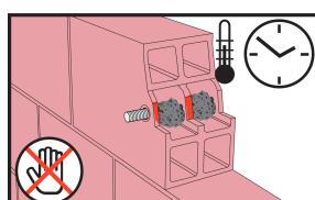
During the resin hardening time the anchor must not be moved or loaded. Wash tools immediately with Sika® Colma Cleaner. Wash hands and skin thoroughly with warm soap water.
