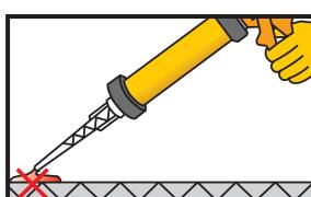
Pump approx. twice until both parts come out uniformly. Do not use this material. Release the gun pressure and clean the cartridge opening with a cloth.
