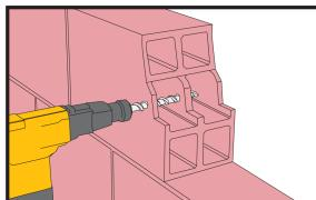
Drilling of hole with an electric drill to the diameter and depth required. Drill hole diameter must be in accordance with anchor-and perforated sleeve size.
