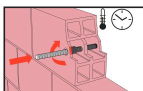
Insert the anchor with a rotary motion into the filled perforated sleeve. Use the adequate steel rod size.
