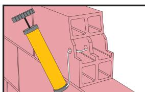
The drill hole must be cleaned after each cleaning step with a blow pump or by compressed air, starting from the bottom of the hole (pump at least 1x).
