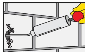
Pump approx. twice until both parts come out uniformly. Do not use this material. Release the gun pressure and clean the cartridge opening with a cloth.
