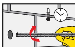
Insert the anchor with a rotary motion into the filled drill hole. Some adhesive must come out of the hole.
