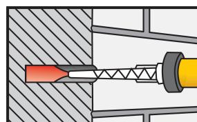
Inject the adhesive into the hole, starting from the bottom, while slowly drawing back the static mixer. In any case avoid entrapping air. For deep holes extension tubing can be used.
