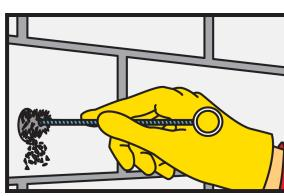
The drill hole must be thoroughly cleaned with the special steel brush (brush at least 2x). The diameter of the brush must be larger than the diameter of the drill hole.
