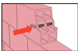
Insert perforated sleeve completely into the drill hole.
