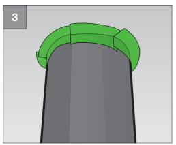
Apply Rissan around circular parts in layers
